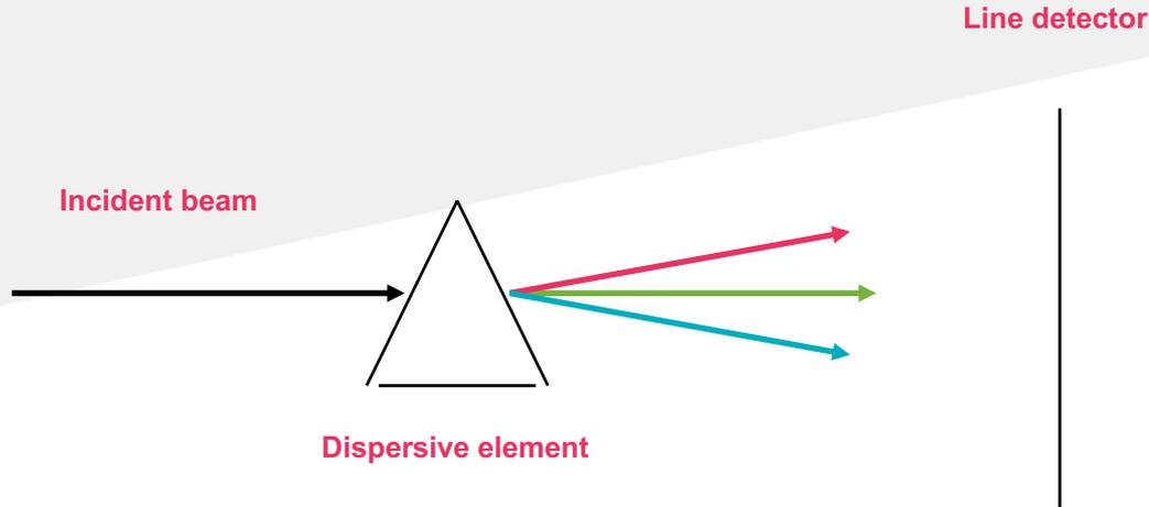
There exist many different means for analyzing the spectral content of the light beam filtered by the pinhole. One of them is the traditional spectrometer, comprising a dispersive element (a grating or a prism) and a line detector.
